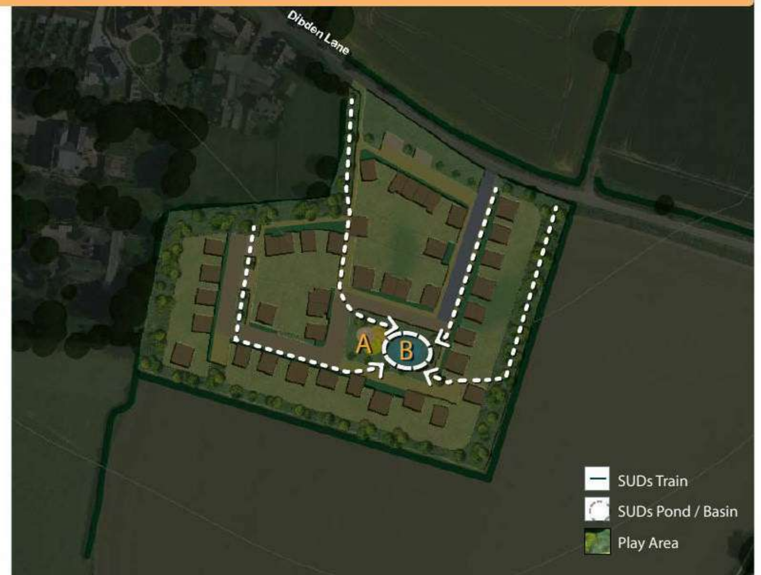
Figure 27: Plan showing SUDs provision across the site, with a SUDs train managing surface water to a SUDs provision in the central open space, via green swales situated along streets and through the open space and landscape belts.
